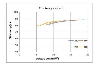
IT FIT 18 220-240 350 CS D L Typical Efficiency vs Load
